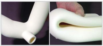
Above: Radiator hose prototype withstands bending without permanent damage or deformation (shown without infiltrant). Left: Primary infiltrant colors of red, yellow and blue can be mixed to create custom colors (black and neutral infiltrants also available).
